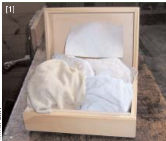
Five different burnishing cloths of varying degrees of coarseness are used
