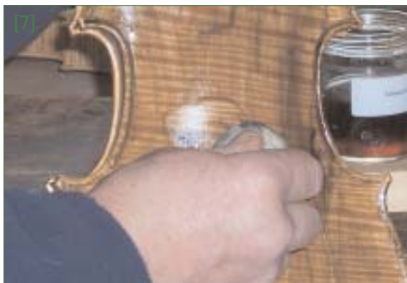
Polishing the surface with the cotton pad dipped in oil and rottenstone
