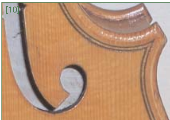
The burnishing method eliminates the haze caused by successive abrasions
