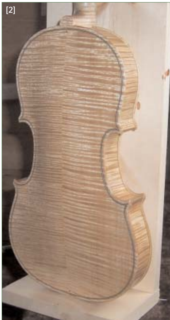
Rubbing with multiple cloths produces a smooth surface ready for varnishing
