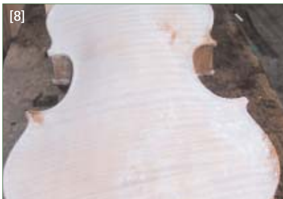
Dusting the surface with flour removes any remaining linseed oil
