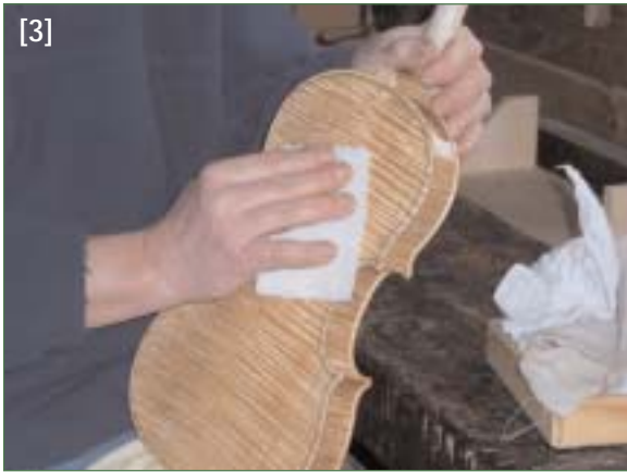
[3] Rubbing with a Scotch-Brite pad removes major imperfections
