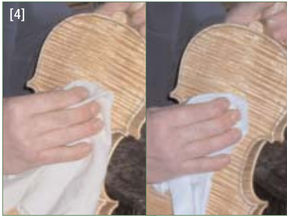
[4] Rubbing continues with a fine linen cloth (left) and a cotton cloth (right)
