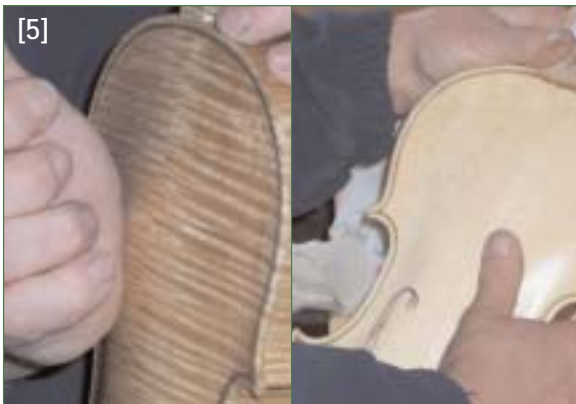
[5] The 'slip' (left) and 'squeak' (right) method shows the time to start burnishing
